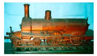
Kyoto University Museum: wooden model of a steam locomotive made in the 1890's The actual locomotive is assumed to be a 2B tender-type (later 5300 type) made by BEYER PEACOCK & CO., LTD imported from England. This passenger locomotive is a classical example used during the middle of the Meiji era, and had no tender coupled to it. In 1893 Japan was at its infancy of railroad technology.
