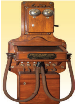
Gowers - Bell telephone
