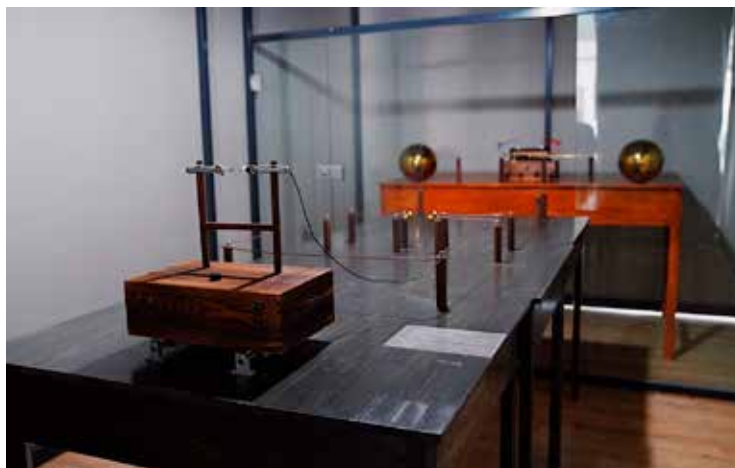
Fig.7 Hertz's experiment restored in ESTM. Image: Wang Nianci
